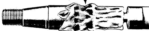
Figure 27 - Grease on Pump Shaft Seals
