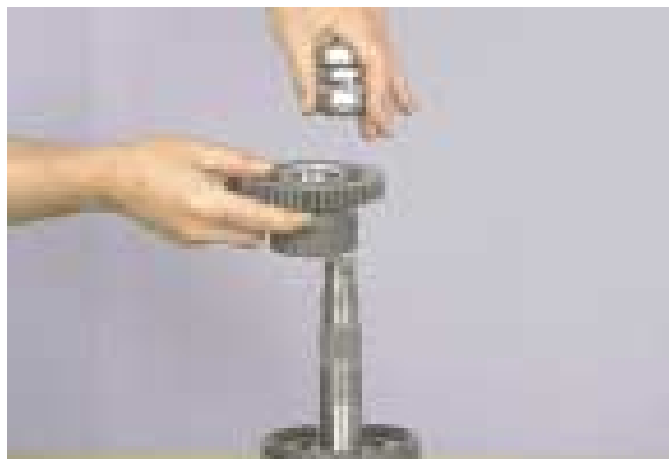
Figure 145 Remove bearings and spacer from clutch gear.
