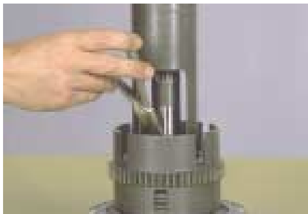
Figure 150 Compress disc springs and remove retainer ring.
