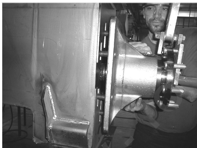
Fig. 5-6 Remove axle housing assembly.
