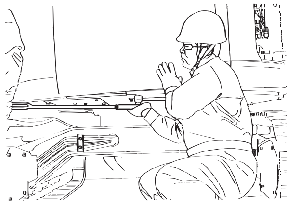
Attaching bolts counterweight
